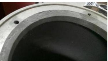
1. Anti-stripping drum, double flange: it is characterized in that the flange of the reducer and the flange of the motor corresponding to the outer wall of the two ends of the drum are respectively provided with a ring of abrupt platform, the clearance between the abrupt platform and the drum is less than the diameter of a traction rope.
